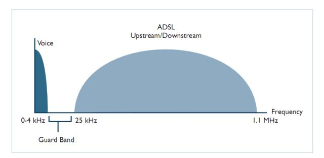
The DSL transmission technology exploits the fact that all voice telephony signals are below 4 kHz in frequency. DSL modems enable up to 1MHz of bandwidth to be used for transmitting digital data alongside analogue (voice) signals on the same wire by band separation of the signals, thereby preventing the signals from interfering with each other. Different operators can use the different paths of the copper wire to provide voice and data respectively.
