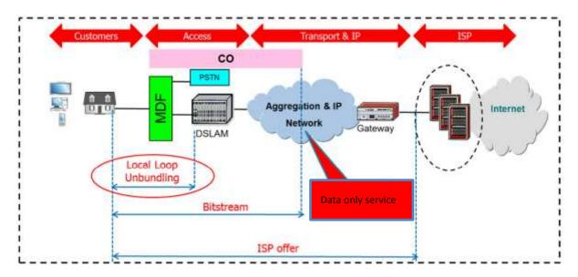
The diagram below illustrates local loop unbundling in a copper network.
