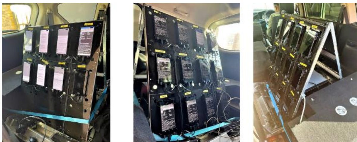
Figure 2. Drive Test System Configuration
